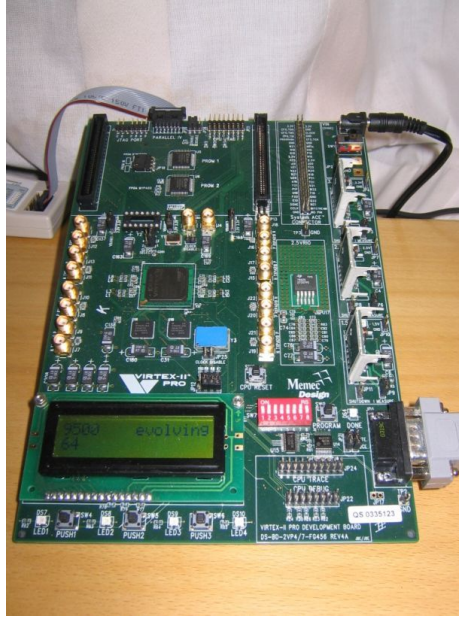
Fig. 1. The prototype board with the Virtex-II Pro FPGA
