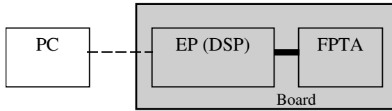
Fig. 1. Block diagram of a simple stand-alone evolvable system
